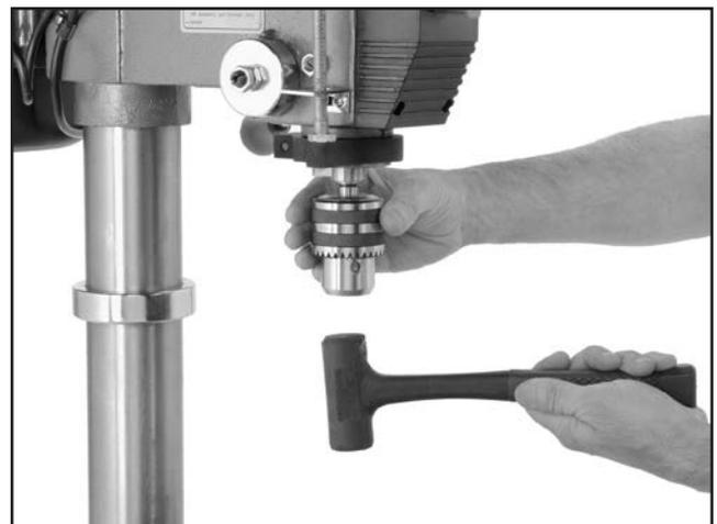
**Figure 16.** Seating arbor and chuck into spindle.
