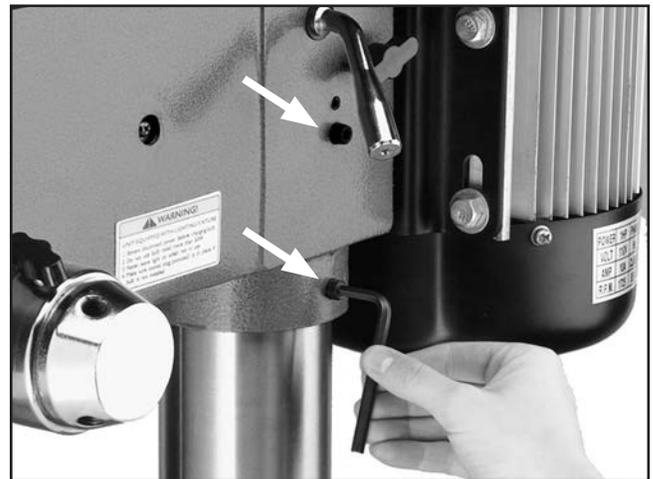
Figure 13. Securing headstock to column.
