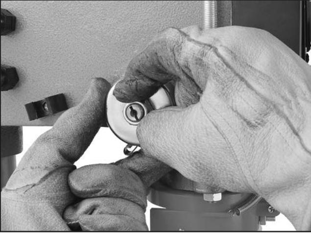
**Figure 48.** Example of loosening cover and jam nut.
