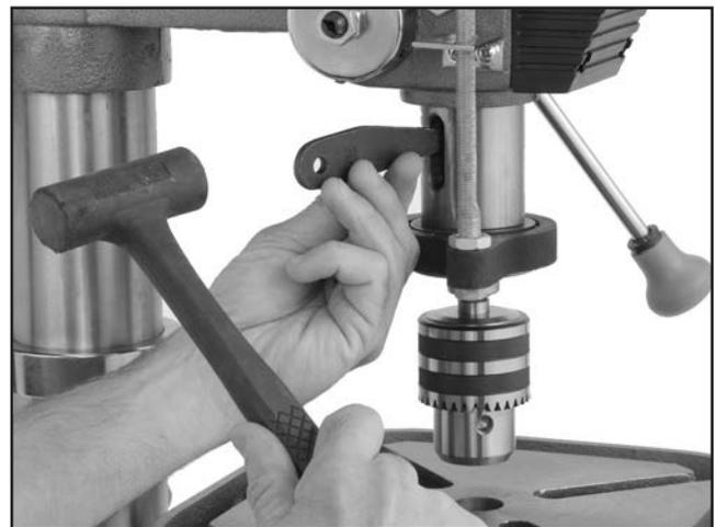
**Figure 33.** Using drift key to remove arbor.
