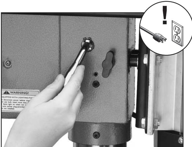
**Figure 27.** Using the belt tension lever.
