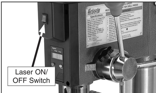
**Figure 1.** Location of laser ON/OFF switch.
