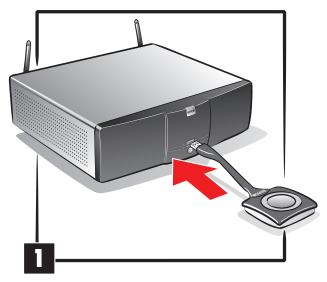
The Button must be paired to the Base Unit before first usage. Insert the Button in the USB port at the front of the Base Unit you are using.
