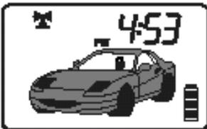
**System Armed** indicates the doors are locked and the Starter Kill is active.
