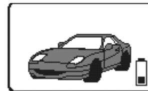
**Battery Low** indicates the battery inside the transmitter needs to be replaced.
