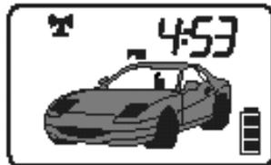
**System Disarmed** indicates the doors are unlocked and the Starter Kill is off.
