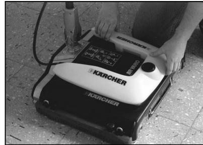
Remove the tank, empty and rinse with water
