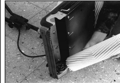
Remove the rotary brushes from the gearing
