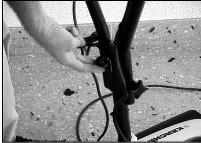
Pull the catch upwards and hold
