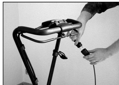
Connect the plug to the power cable
