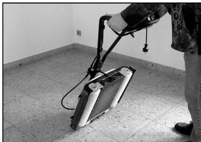
Push the appliance onto the track rollers
