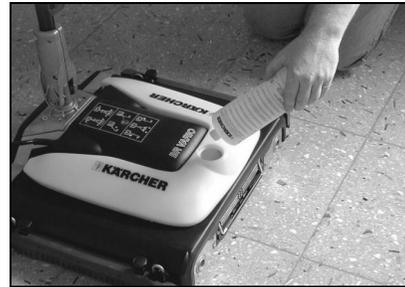
Fill the tank with the required amount of cleaning agent
