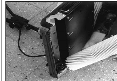
Place the rotary brush with gearing onto the drive
