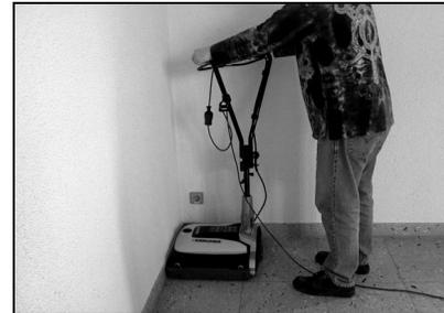
Press the pushing handle downwards and turn to the LEFT or RIGHT
