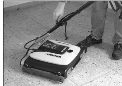
Release the pushing handles and tip forwards
