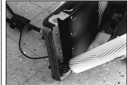
Remove the rotary brushes from the gearing
