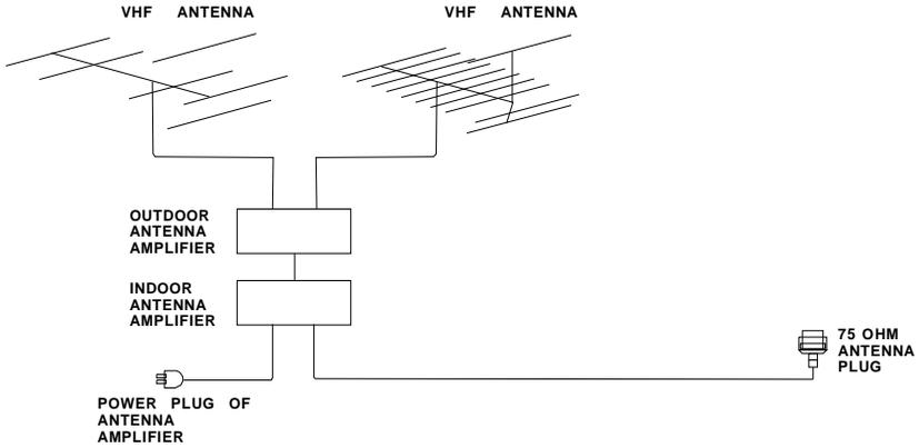
To ensure good picture and sound, TV antenna system needs to be installed. The antenna system as shown can be sourced from TV equipment shops, which will provide service for correct installation and connection. After installation, insert the 75-ohm antenna plug into the antenna jack as shown. In case of signal of closed circuit TV,
