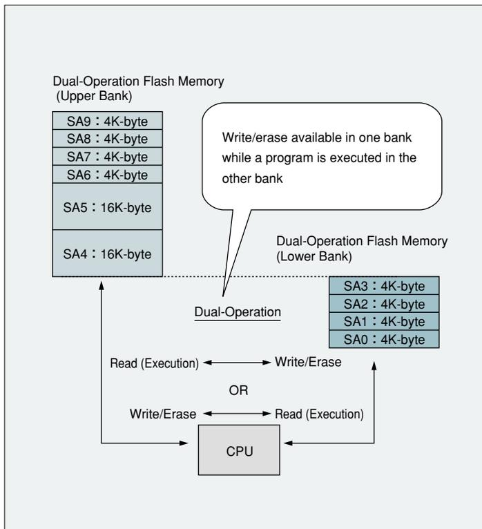
Figure 2 Operational Flow of CPU Rewrite by Flash Memory
