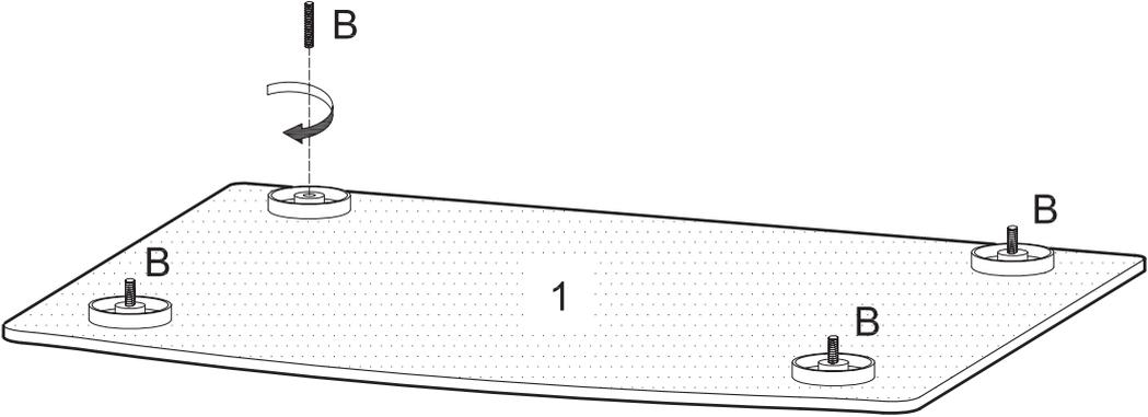
Carefully lay glass top (1) upside down on a soft surface. Screw short rods (B) into the metal plates of glass top (1).
