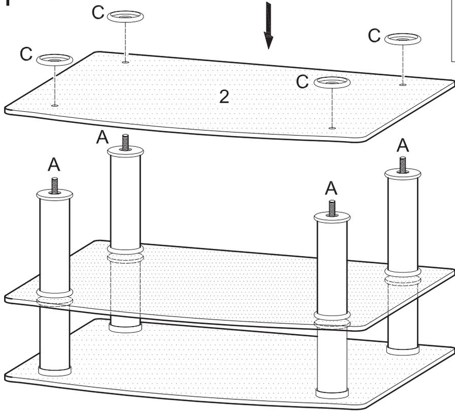
Carefully lay glass shelf (2) in place using long rods (A) as guides. Place decorative rings (C) over long rods (A).
