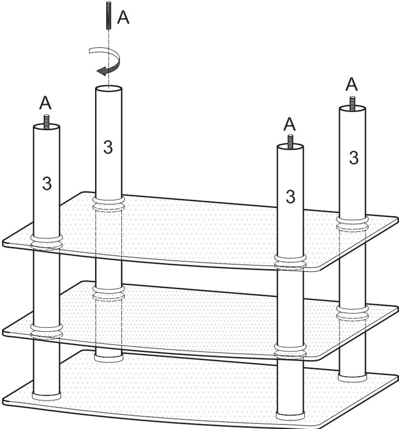
Screw long rods (A) into cylinders (3).
