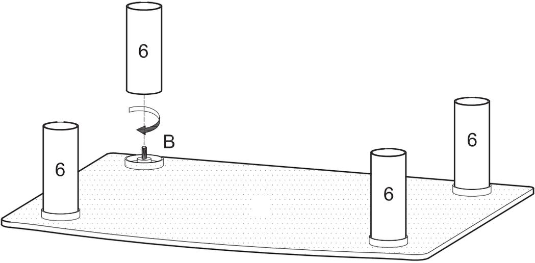
Screw cylinders (6) onto short rods (B).
