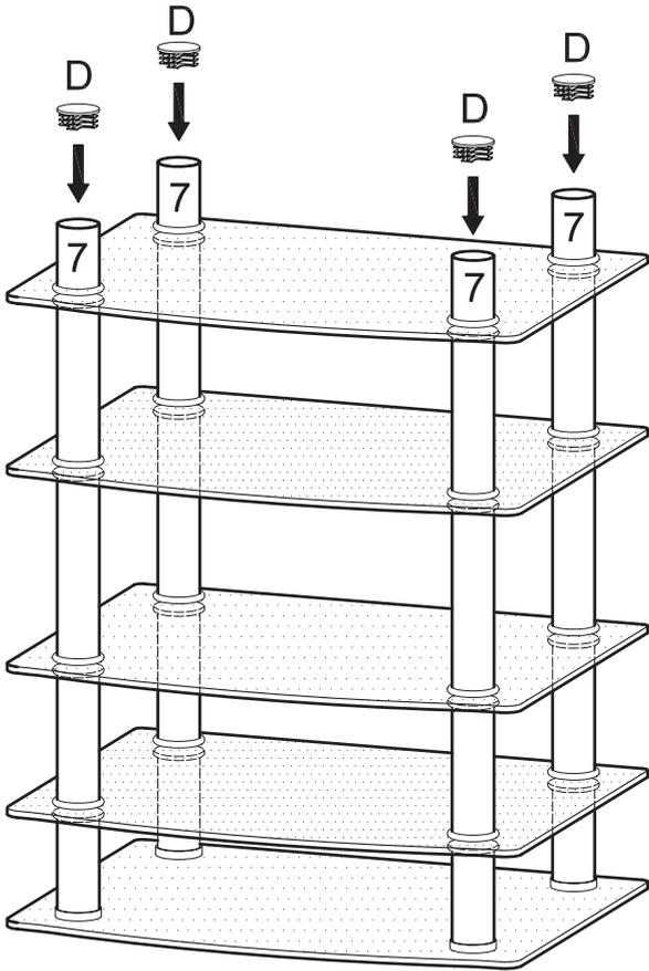
Insert caps (D) into cylinders (7). Note that caps (D) may come pre-inserted into cylinders (7).
