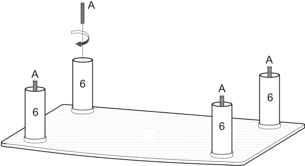
Screw long rods (A) into cylinders (6).
