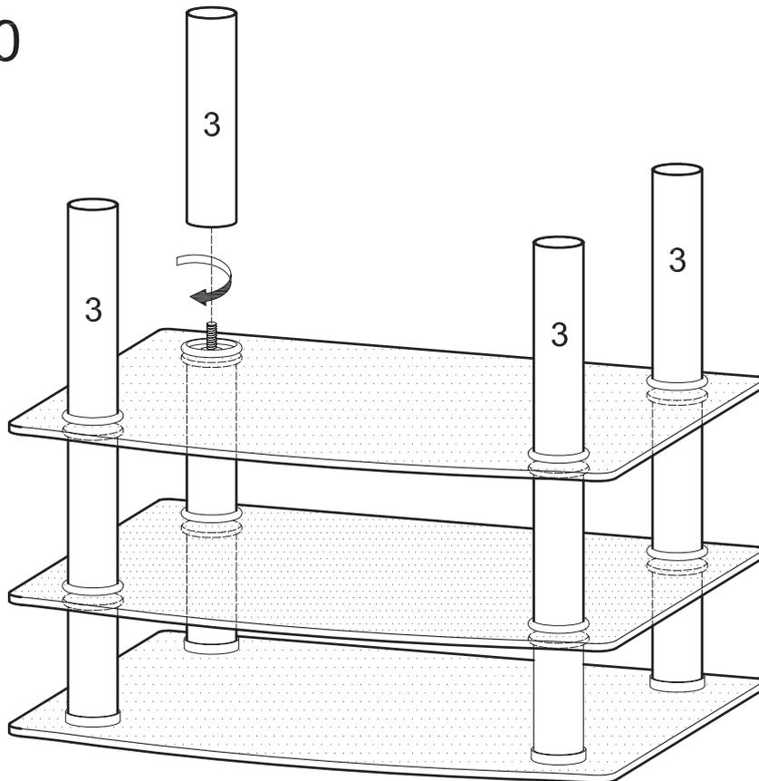
Screw cylinders (3) onto long rods (A). Note that cylinders (3) will fit snugly inside the decorative rings placed in the previous step.
