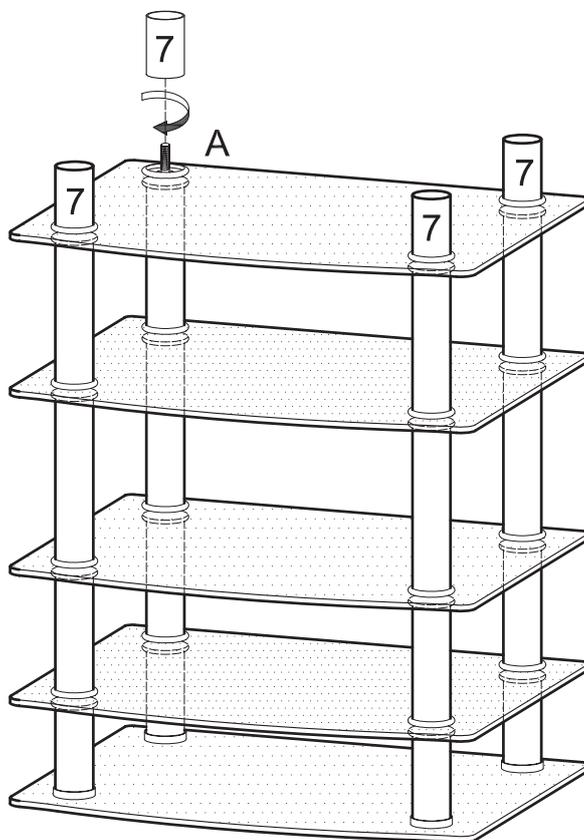
Screw cylinders (7) onto long rods (A). Note that cylinders (7) will fit snugly inside the decorative rings placed in the previous step.
