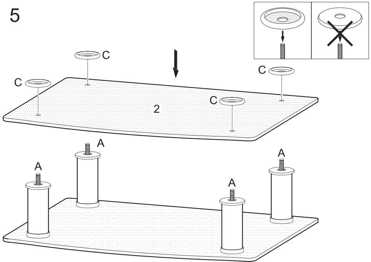
Carefully lay glass shelf (2) in place using long rods (A) as guides. Place decorative rings (C) over long rods (A).
