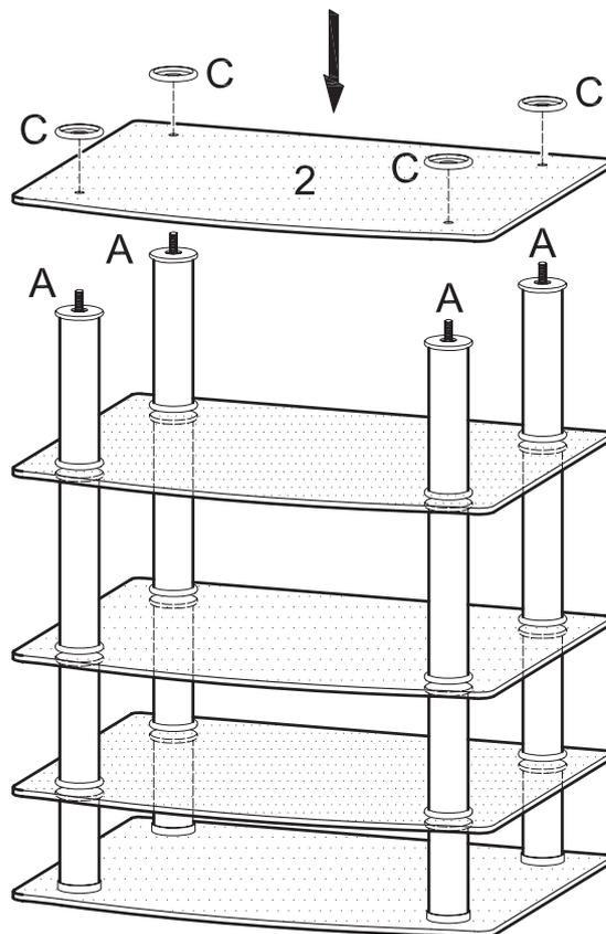
Carefully lay glass shelf (2) in place using long rods (A) as guides. Place decorative rings (C) over long rods (A).
