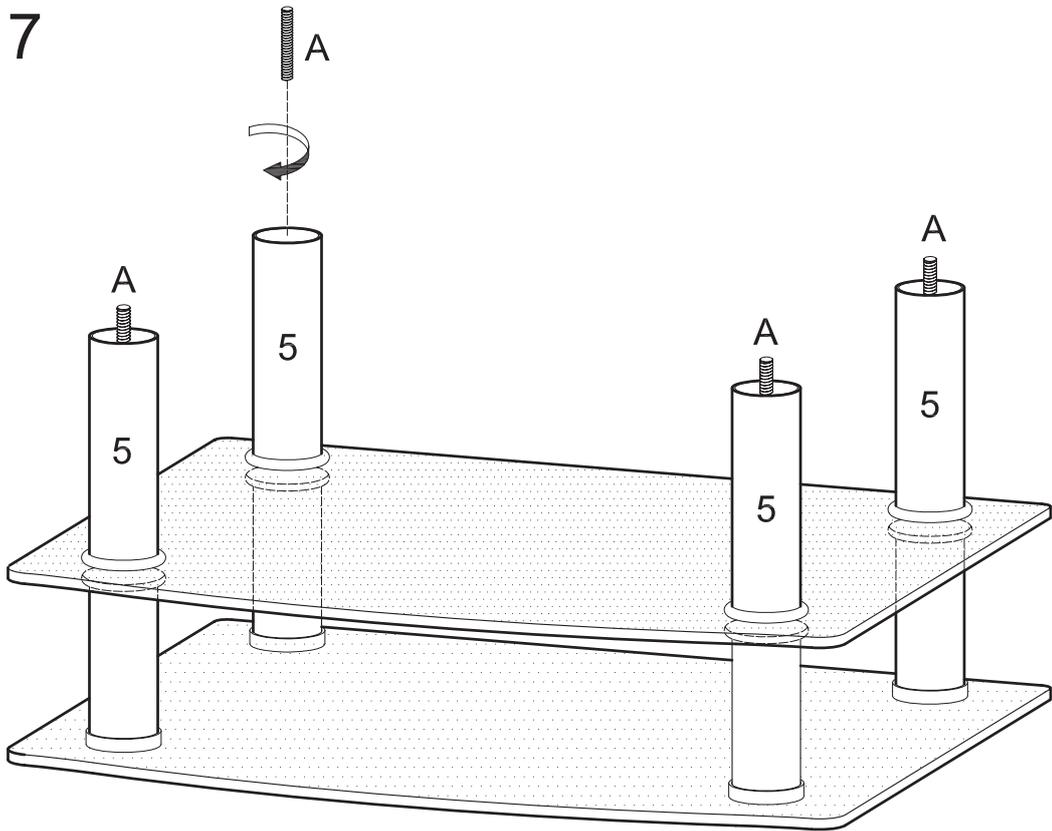
Screw long rods (A) into cylinders (5).
