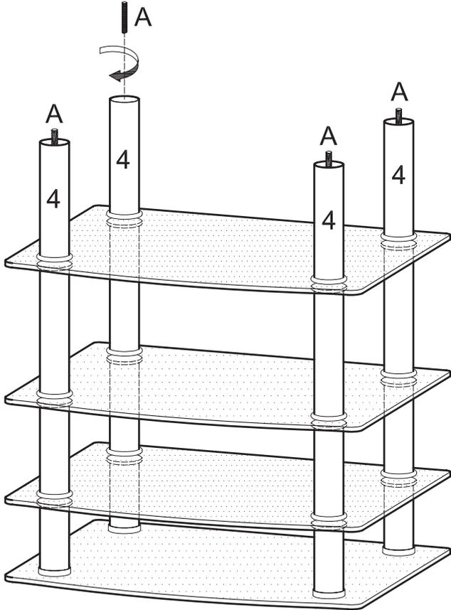
Screw long rods (A) into cylinders (4).
