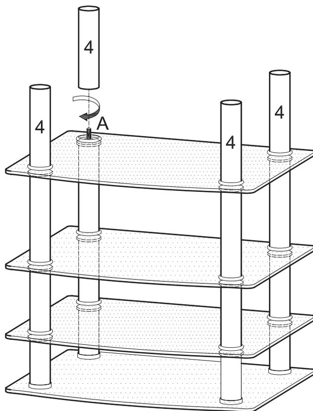
Screw cylinders (4) onto long rods (A). Note that cylinders (4) will fit snugly inside the decorative rings placed in the previous step.
