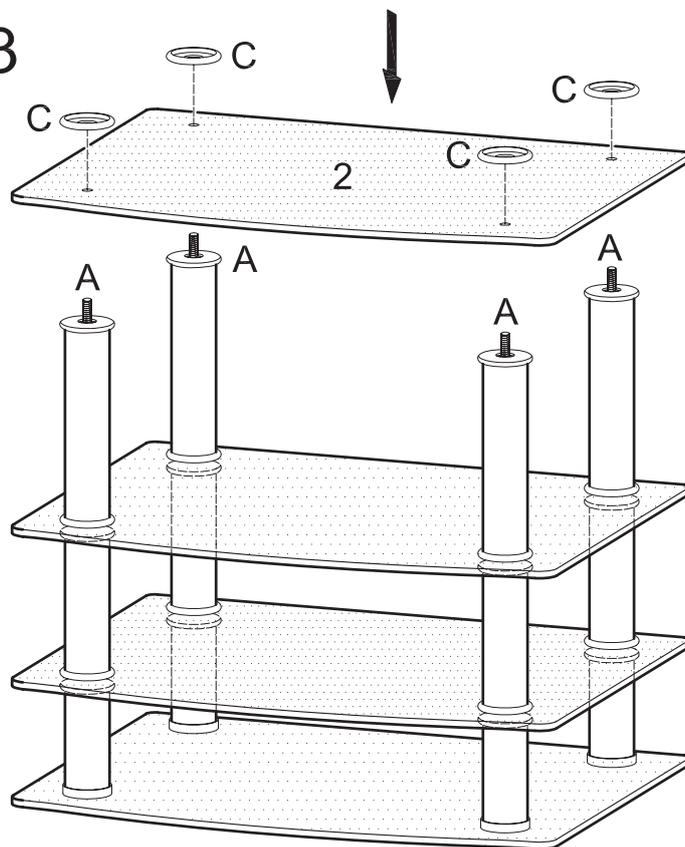
Carefully lay glass shelf (2) in place using long rods (A) as guides. Place decorative rings (C) over long rods (A).
