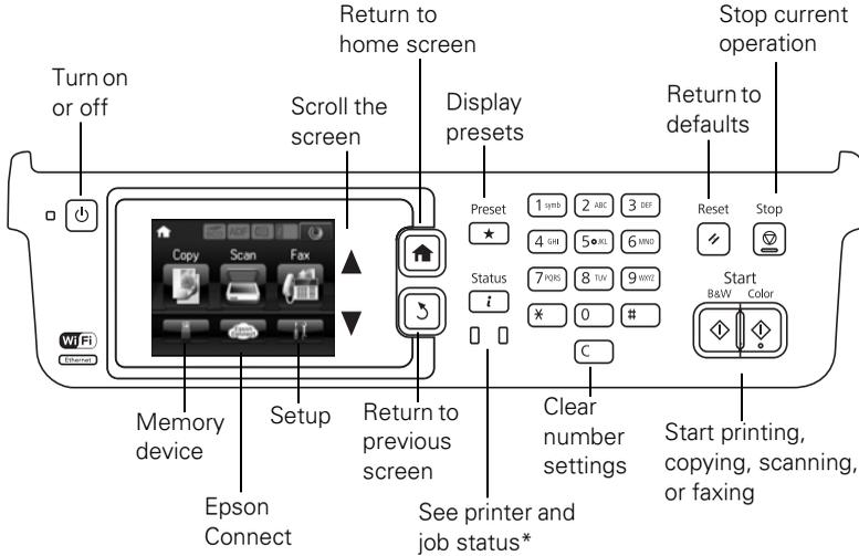
\* The orange light (on the left) comes on when a cartridge is low on ink. It flashes when an error occurs or a cartridge is expended. The blue light (on the right) comes on when there are jobs waiting, and it flashes when the product is processing data.
