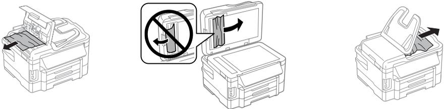
At the back of the printer, remove the auto-duplexer (rear cover), and check these areas:
