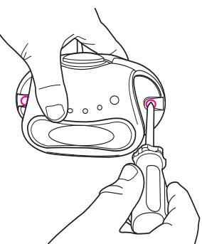
Remove 2 screws from back of electronics module.
