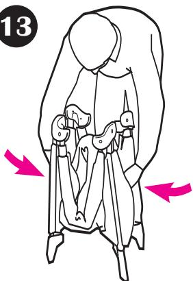
**Do not force.** If unit will not fold, look for a partially latched top rail. Squeeze the latch button to release the rail.
