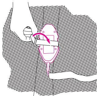
Vibrator must be fastened tight and centered on the webbing strap to work properly.
