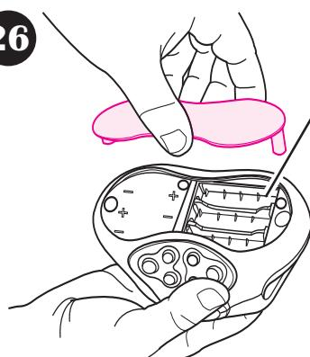
Remove battery door and insert 3 "AA" batteries. Replace door and screws.
