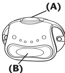
**LIGHTS**— Press once to turn top light **(A)** on, press twice to turn both lights on, press three times to turn bottom light **(B)** on, and four times to turn lights off.
