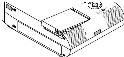
3. Remove the lamp housing by pulling out the handle.
