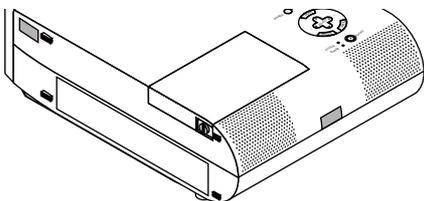
2. Loosen the two screws securing the lamp housing until the screwdriver goes into a free-wheeling condition. The three screws are not removable.
