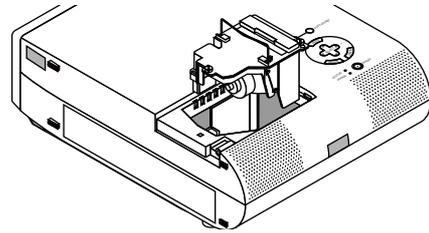
5. Secure it in place with the two screws.
