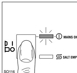
Close the door and depress the ON/OFF pushbutton. The pilot light will come on and the machine will start. If you wish to interrupt the wash at any time press button again.
