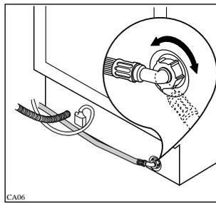
**Note:** the end of the hose connected to the machine can be positioned as required, by simply slackening the retaining ring.
