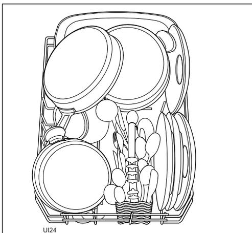
Cutlery should be placed in the removable cutlery basket with the handles facing downwards. If the handles protrude from the bottom of the basket, obstructing the lower spray arm, load the cutlery with the handles facing upward.
