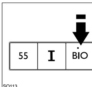
When the "BIO" button is depressed, any prewash is with cold water and the main wash at 50°C, suitable for compact and tablet detergents containing enzymes.
