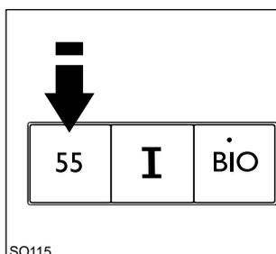
When the "55" button is depressed, any prewash is with cold water and the main wash at 55°C.
