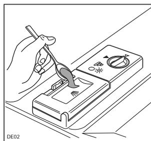
All the programmes with prewash required a small extra amount of detergent of approximately 5 g (10 g for the Intensive programme) to be poured over the dispenser's lid as shown in the picture.
