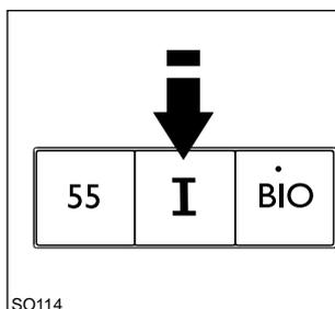
When the 'I' button is depressed, the prewash is at 55°C and the main wash at 70°C.
