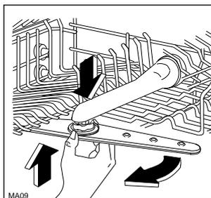
Slide out the upper basket. Push downwards on the water feed pipe, simultaneously push the spray arm upwards and turn it in a clockwise direction.
