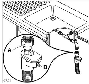
The problem is signalled by a red indicator which appears in window (B). If this happens, close the water tap and have the hose replaced.
