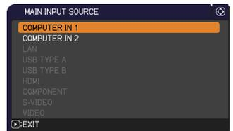
**NOTE** • When FIXED (COMPUTER IN 1) is selected, the MONITOR OUT setting is invalid. ([Operating Guide](#) → [SETUP menu](#))
