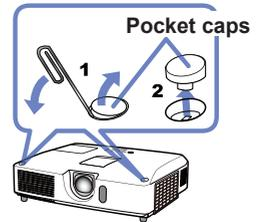
**NOTE** • Cap storage pockets for the pocket caps are inside the lens adjuster door. Be sure to keep the caps in the storage pockets after removing the caps from the stack pockets.
