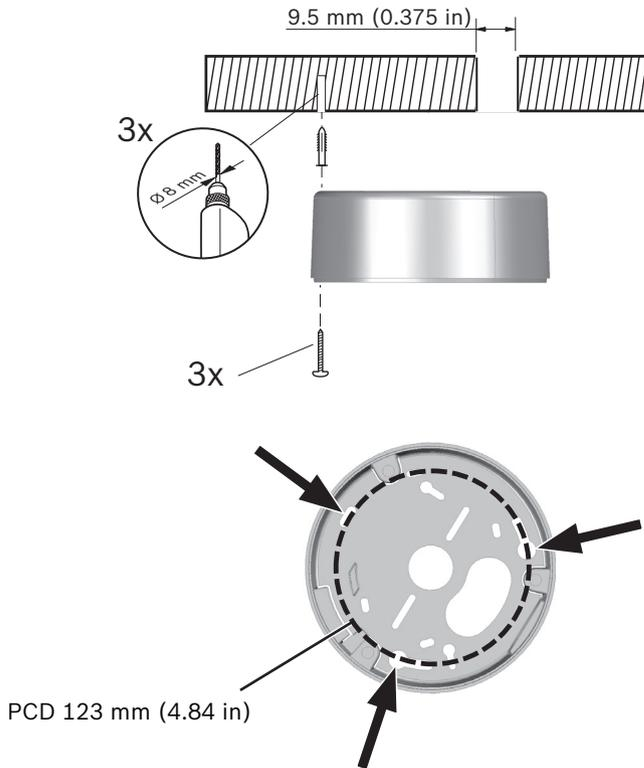
To mount the camera on the surface of a wall or ceiling:
