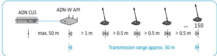
The transmission range of the antenna module and the wireless conference units is approx. 30 m. The transmission range can vary depending on location and environmental conditions such as wall thickness, wall composition etc.
