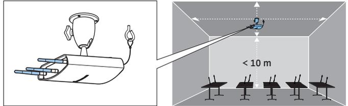
Wall mounting is recommended for rooms with a ceiling height of more than 10 m because the wireless conference units have an omni-directional radiation pattern (approx. 30 m):
