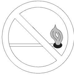
Fig. 3 - Do Not Light Burner with Match
