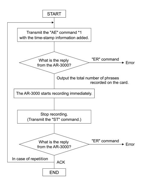
\*1 Setting such as RDAC-Grade and RDAC-Mode are made by "AE " command parameters.
