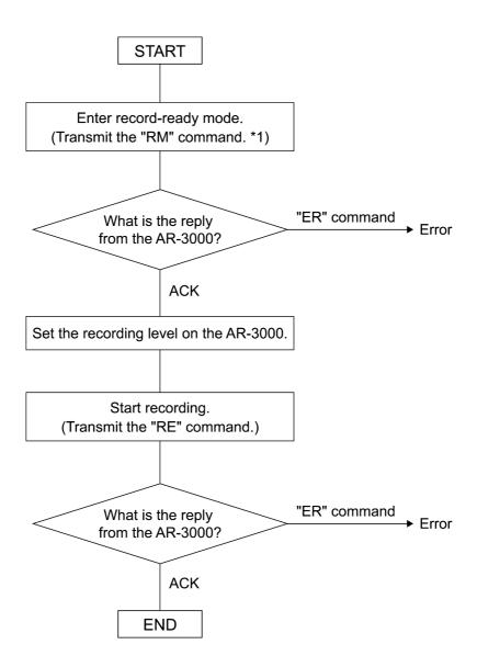
\*1 Setting such as RDAC-Grade and RDAC-Mode are made by "RM" command parameters.
