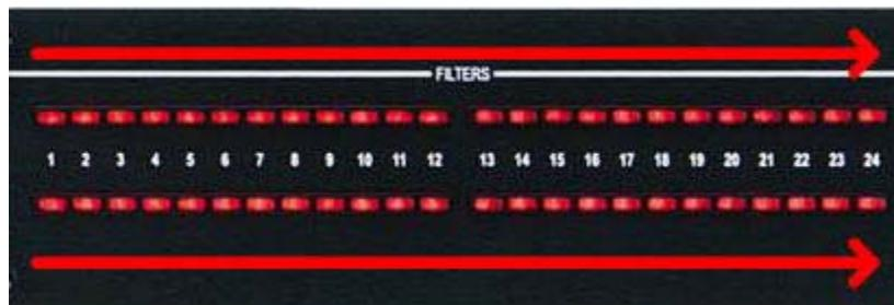
3. The Mode buttons should be lit a yellow or amber color. If they are not press each **MODE** button until they are both yellow. The filter LEDs will indicate how many total filters will be active.
