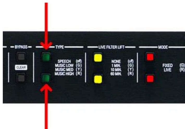
18. If you find that the feedback reoccurs when the Live filters are lifted, try setting a longer Live Filter Lift time or try setting it to “None” (LED off).
