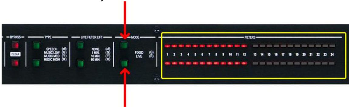
Press the **LIVE FILTER LIFT** buttons to increase the # of “Fixed” filters for each channel. Press the **TYPE** buttons to decrease the # of “Fixed” filters for each channel.
