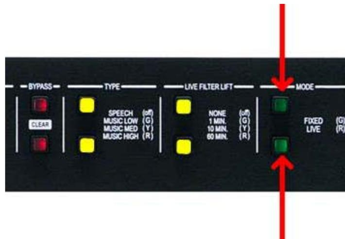
14. Disengage the Bypass buttons (LEDs off).
