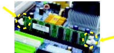
1. The DIMM slot has a notch, so the DIMM memory module can only fit in one direction.
