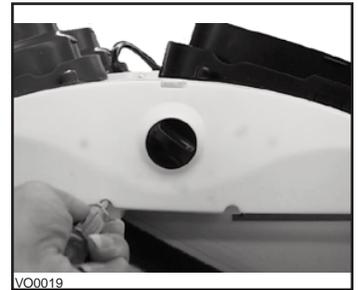
9. Using a small rod, pierce a hole through the unit at the end of the wire channel in front of the unit. (See picture beside.) Splice back the end of the cable to access the 4 wires. Remove the insulated sleeve of each wire ends. Insert the end of the cable through the unit, using the small hole previously done. From the top right front hole of the unit, pull on the wire.
