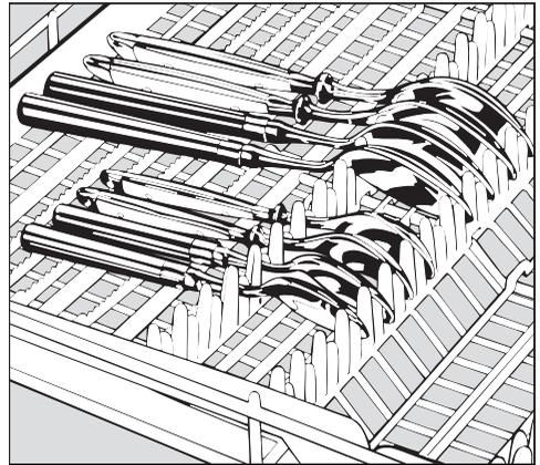
Spoons with thick handles may have to be placed as knives and forks with their heads in the holders.
