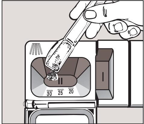
The horizontal marks in Compartment II indicate levels of approximately  $1\frac{1}{4}$ ,  $1\frac{3}{4}$  and 2 tablespoons (20, 25 and 30 ml) respectively.
