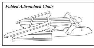
Secure folding mechanism forward into stationary position with chair in upright position.
