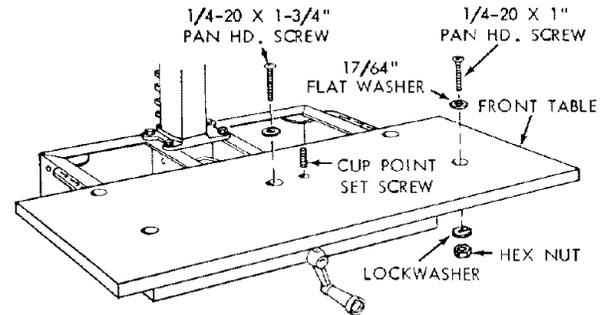
4. Lay the rear table board on edge across the front table to serve as a straightedge. Sight under this straightedge to determine whether the front table board is high or low at its center.
