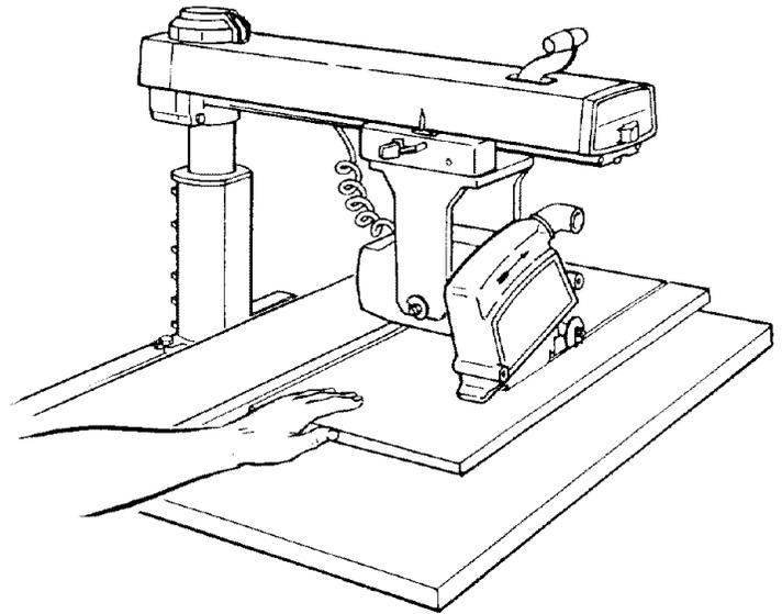
**In-Ripping.** The radial arm and bevel are indexed at 0° and locked, but the yoke is turned 90-degrees in a clockwise direction (viewed from above) from the crosscut position. Thus, when standing in front of the saw, the blade would be rotating counterclockwise. After positioning the guard and antikickback mechanism the workpiece is fed from the right-hand side of the saw. The "Blade In-Rip" scale is on the right-hand side of radial arm.
