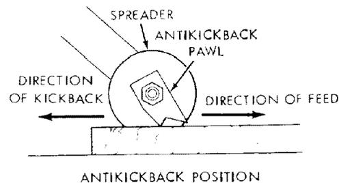
3. Loosen the wing screw and with the tab provided, position the antikickback and spreader assembly until the pawl assumes approximately the position shown above. Tighten the wing screw.
