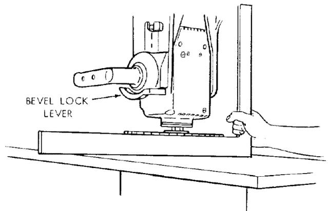
3. If the saw blade is parallel with the table top (no visible gap appears between the saw blade and square), no adjustment is required.
