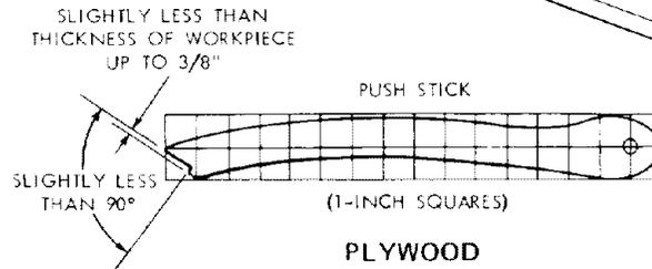
7. When ripping stock 1/4 inch or less between the blade and fence (guide) use a Pusher Board.
