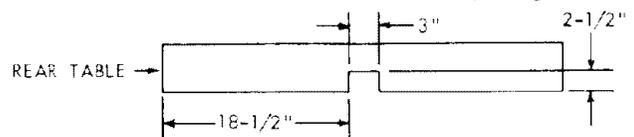
For top-side rabbeting or molding in the in-rip position, relieve the fence by positioning the cutting tool at the desired location on the arm, locking the Carriage Lock Knob, and lowering the cutting tool slowly into the fence – remove only as much material from the fence as is necessary.
