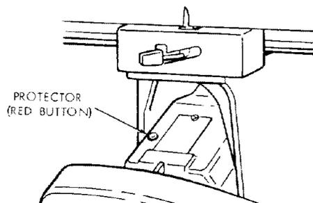
1. If the protector opens the line and stops the saw motor, immediately press the saw switch to the "OFF" position, and allow the motor to cool.
