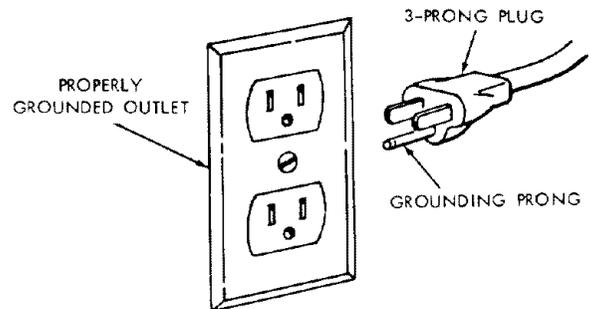
This power tool is equipped with a 3-conductor cord and grounding type plug which has a grounding prong, Listed by Underwriters' Laboratories. The ground conductor has a green jacket and is attached to the tool housing at one end and to the ground prong in the attachment plug at the other end.
