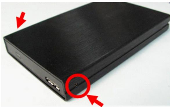
6. With the enclosure fully assembled, connect the USB 3.0 cable from the enclosure to a USB port on the host computer system using the included cable.
