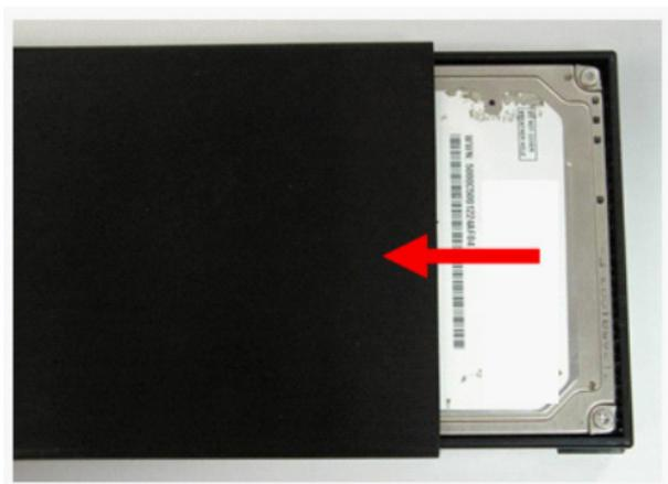
5. Mount the Hard Drive Tray to the Metal Enclosure by inserting 2 of the smaller included screws into either side of the enclosure. Fix them into place using the included Screw Driver.
