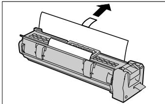
7. Insert the cartridge as shown below and slide it into the machine until it clicks.
