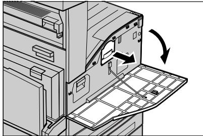
3. Hold the handle and remove the cartridge from the machine.
