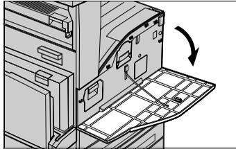
2. Open Tray 5 (Bypass) and then Cover A while lifting up the release lever.
