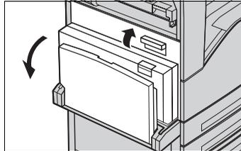
3. Lift up the colored lever, and slide the drum cartridge out until you can grasp the handle on top of the cartridge.
