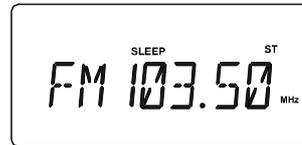
When the Sleep Timer counts down to "00", the power shuts off automatically.
