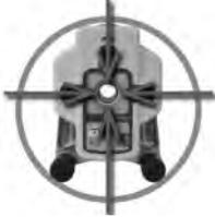
**Automatic-Spot-Match:** (like Grade Match- two existing elevation points will be connected to measure the grade value between these two points) aligns the plumb beam automatically to the SF601 center point (both axes) and moves back to Z-axis automatic mode while displaying the measured Z-axis grade value.
