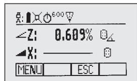
4. When Spot Match has been completed, the fan beam will be turned off and the UL calculates the grade value between both elevation points. The calculated grade value will be displayed at the UL's and RC's display.
