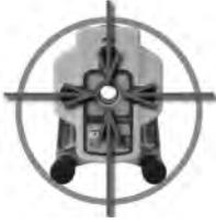
Using **SpotLok mode** (like PlaneLok) aligns and holds the plumb beam automatically to the SF601 center point (both axes) until exiting this mode.
