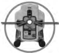
**Automatic-Spot Alignment:** SF601 guides the beam to the target point in the horizontal axis, while the Z-axis grade value will be maintained. Used for first and second day alignment (pipe laying applications).
