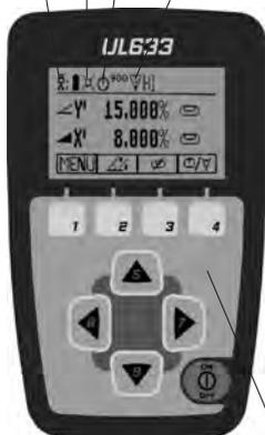
**Button 1:** Quickly press and release starts the **MENU** entry.
