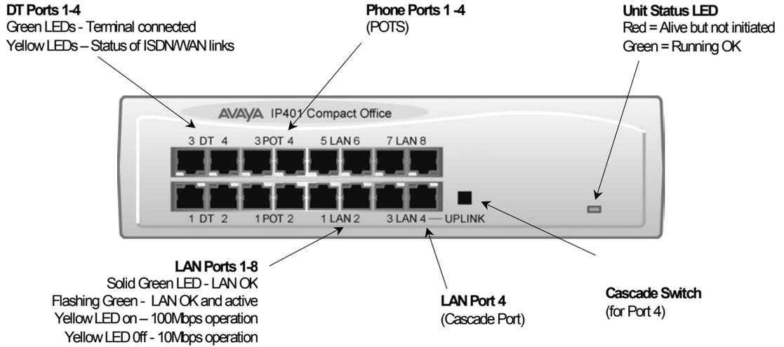
**Note:** The IP Compact Office DT4 is shown above. The IP Compact Office DT2 does not have the top row (labeled **3 DT 4**, **3 POT 4**, **5 LAN 6** and **7 LAN 8**) of RJ45 ports fitted.
