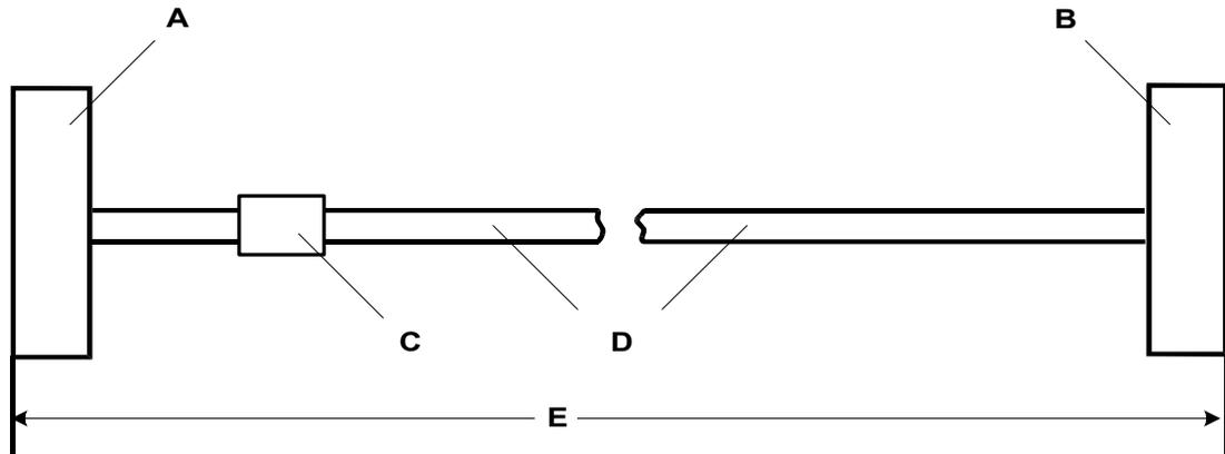
A 37 Way D-Type Plug with UNC 4-40 locking screws.
