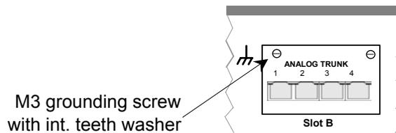
2. Connect, using a fastening that satisfies local regulations, the other end of the wire to the approved round, such as building steel or a cold water pipe.
