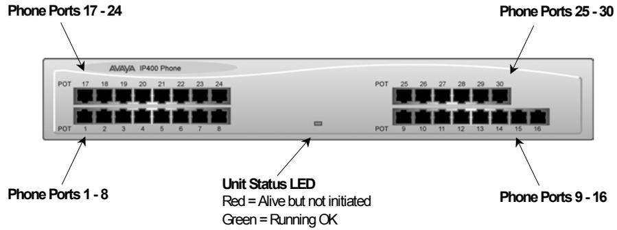
**Notes:** The IP400 Phone 8 variant is only equipped with the bottom left row of ports. The IP400 Phone 16 variant is only equipped with the bottom row of ports.
