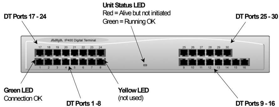
**Note:** The IP400 Digital Terminal 16 Expansion Module is only equipped with the bottom row of ports (1-16).
