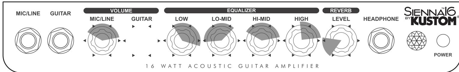
Standard Single Input Setup - in this setup your acoustic/electric guitar is plugged into input 1. (Remember, if you are using an active guitar or pre-amplified guitar, you may need to lower the guitar's volume control if you encounter distortion. We suggest that you turn its output level to about mid-way up and this will give you a cleaner sound as well as giving you available headroom for leads.) The tone controls follow both inputs.
