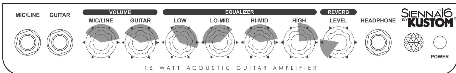
Standard Dual Input Setup - in this setup two inputs are utilized. Guitar is plugged into guitar input jack and a Hi-Z microphone is plugged into mic/line Input. Assuming you are also using a microphone, plug it into the mic/line jack and slowly turn up the mic/line volume control. Balancing the two types of inputs gives you a much more natural acoustic guitar sound.
