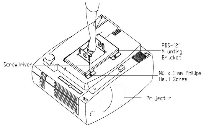
1. Invert the projector and place it on a soft and flat surface. Remove any foot levelers that might possibly prevent the correct installation of the bracket.
