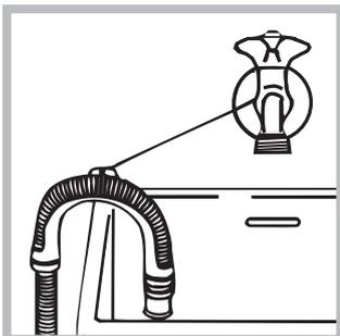
If it is place over the edge of a basin or sink be sure the free end of the hose should not be underwater.
