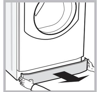
1. take off the cover panel on the front of the machine by first pressing it in the centre and then pushing downwards on both sides until you can remove it (see figures);
