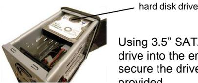
Using 3.5" SATA hard disk drives, slide the drive into the embedded drive bay and secure the drive to the bay with screws provided.
