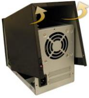
Loosen the 3 screws at the back of the tower using a Philips screwdriver by turning counter-clockwise. Separate the metal casing of the storage tower from the housing by lifting up the casing as shown on the photo.
