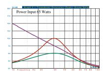
with the filter and with the filter and the INTELLi Q set to +3dB. As you can see with +3dB of boost and the high-pass filter set to 30Hz, the woofer has more output down to 25Hz and less overall excursion when compared to the non-high-pass response. Maximum physical excursion capability of the woofer is 15mm.
