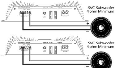
**SYSTEM** 5 has one amplifier driving front satellites, one amplifier running as a Master Amplifier and additional amplifiers running as Slave amplifiers to the master. The subwoofer amplifiers are configured in a Master/ Slave configuration for absolute crossover and level matching.
