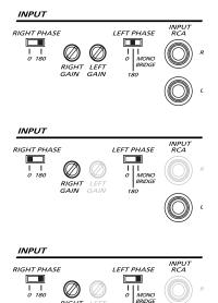
Setting 4 inverts the output of both the left and right channels. Both left and right gain controls are active. This configuration is useful for inverting one set of speakers like rear speakers in front/rear system to improve staging in a vehicle.
