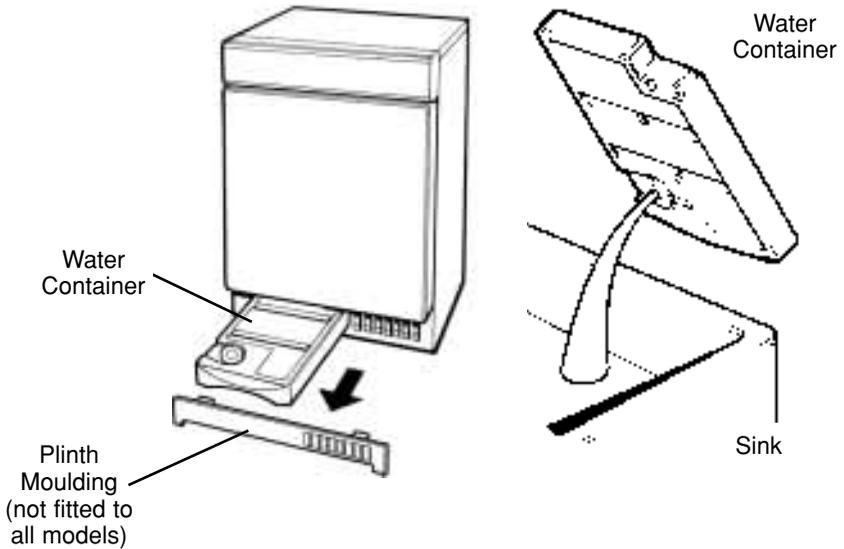
**Empty the water container after EVERY programme. Failure to do this will result in the water container becoming full and the load will not dry.**
