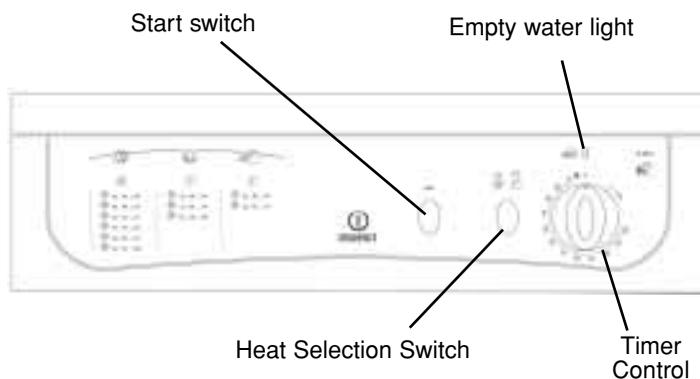
**Setting the timer** The drying time for both heat settings is controlled by the timer. All you have to do is turn the Timer Control **clockwise** until the required time appears in line with the indicator.
