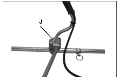
11. Secure throttle linkage and leads to drive shaft with cable clips supplied.
