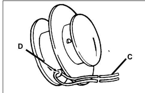
3. Hold the spool, opening toward you. Place index finger between the two strands and wind line, tightly and evenly, in direction of arrow marked "CC".
