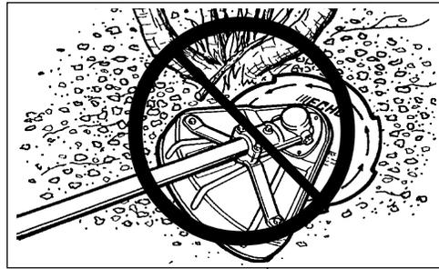
**Brush/Clearing Blade P/N 69500120331** is designed for cutting brush and woody growth up to 76 mm (3" in.) diameter.
