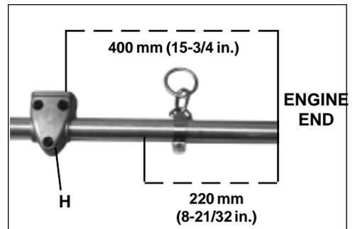
10. Install upper U-Handle and bracket on lower bracket and secure with one (1) 8mm x 55mm bolt (J) and large circular washer.
