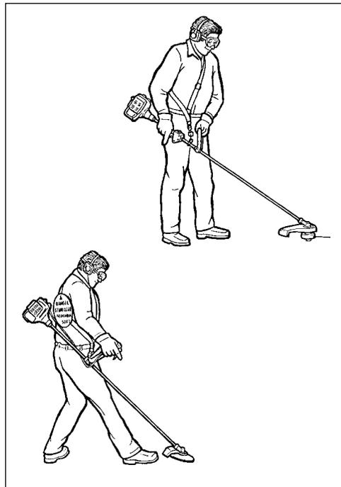
During blade operation, the same fatigue reduction is achieved. Safety to the operator is also enhanced by preventing blade contact with the operators hands and feet by restricting trimmer movement.
