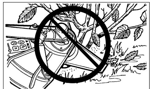
**8 Tooth Weed/Grass Blade P/N 69600120331** is designed for grass, garden debris and thick weeds. **DO NOT** use this blade for brush or heavy woody growth, 3/4" in. (19 mm) diameter or larger.
