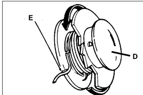
4. Stop when approximately 15-20 cm (6-8 in.) line (C) remains and place ends of line in notches (E) in spool (B).
