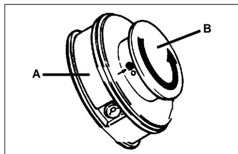
8. Pull both lines out and trim to cut-off knife length.
