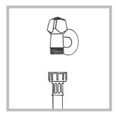
1. Connect the inlet hose by screwing it to a cold water tab using a 3/4 gas threaded connection (see figure).
