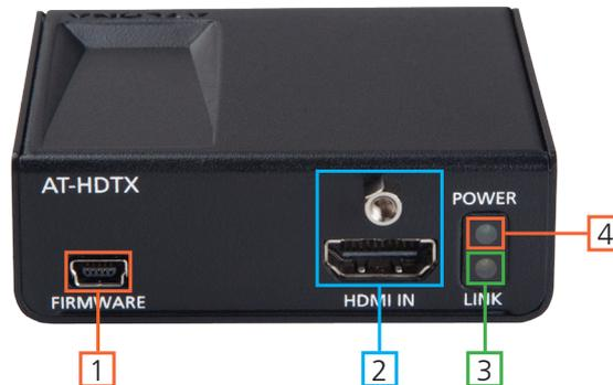
1. Firmware Update Port: Use Mini USB to USB cable to connect to a Windows computer to update.
