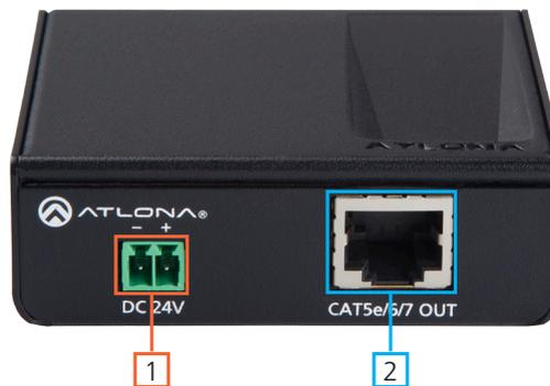
1. Power Port: Connect included captive screw connector and power adapter here.
