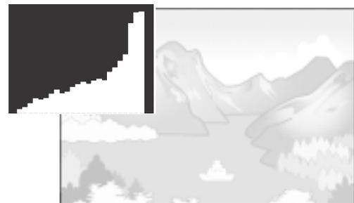
If the histogram has only peaks on the left side without anything else, this picture is under-exposed with too many pixels only for shadow sections.
