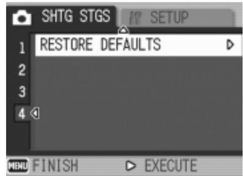
The display indicates the camera is restoring the initial settings; once it is finished, the display returns to the Mode screen.
