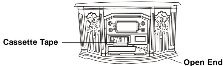
**Note:** There is no 'TAPE' position on the Function selector. When you insert a cassette onto the player the system automatically switches to the Tape mode.
