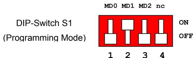
Figure 3-2: MCU mode switch: Flash Programming mode
