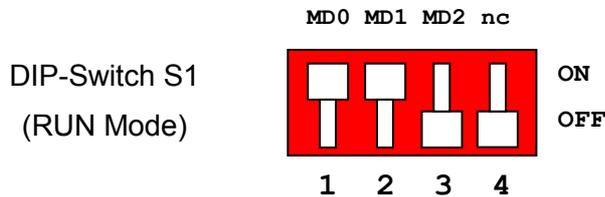
Figure 3-1: MCU mode switch: RUN mode (Fixed Vector Mode)
