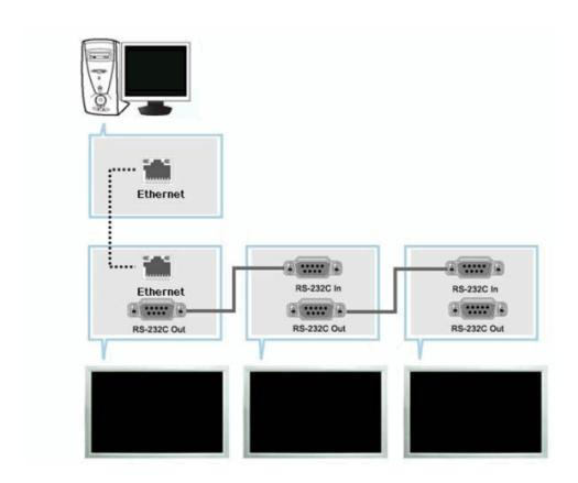
Unlike the previous method which used the serial data communication specifications RS-232C, an Ethernet function has been added.
