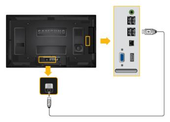
1. Connect the [TOUCH SCREEN USB HUB] port of the product to the USB port on your PC using the USB cable.
