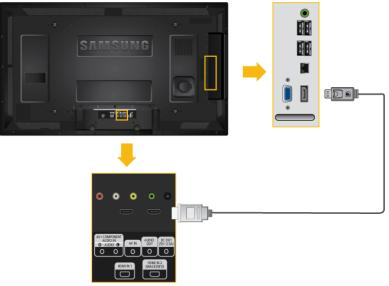
Connect the [MAGICINFO OUT] terminal of the network box and the [HDMI IN 2 (MAGICINFO)] terminal of the monitor using the DP to HDMI cable.
