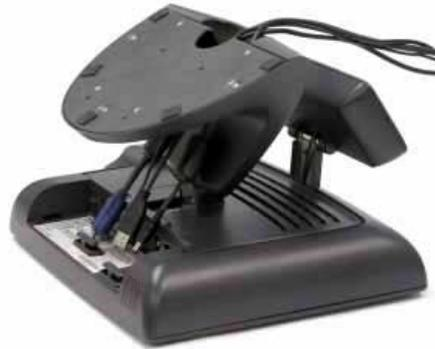
**NOTE:** Before connecting the cables to the touchmonitor, route all the cables through the hole in the stand as shown in the picture above.
