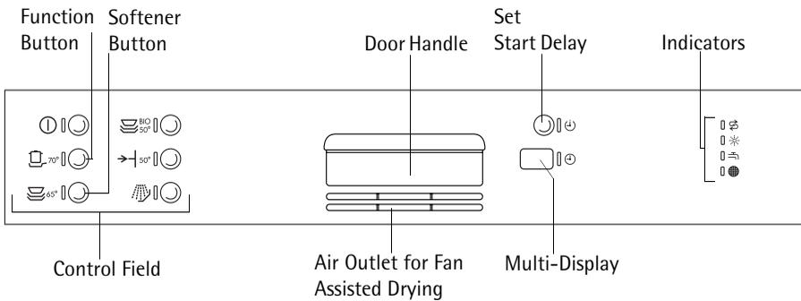
The **Control Field** comprises the ON/OFF switch (⏻) and the programme buttons with LED indicators.
