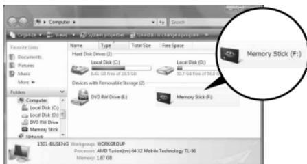
This “Memory Stick (F:)” indicates this unit is inserted into the computer. Depending on your computer, the drive name ((F:) etc.) may differ.
