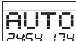
turn on the fan at high speed, press the button a second time; the word "HIGH" will appear in the matrix. To select the auto mode, press the button again; the word "AUTO" will appear in the matrix. When the auto mode is selected, the speed of the fan will automatically increase and decrease as the speed of the walking belt increases and decreases.
