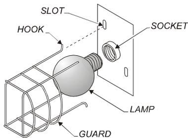
3. Unthread old heat lamp from its socket and discard.
