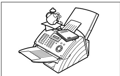
Do not place heavy objects or spill liquids on the machine.
