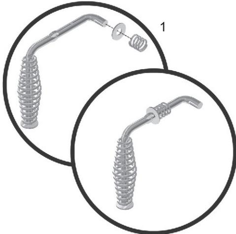
1. Slide the handle washer onto the end of the door handle, followed by the handle spring.
