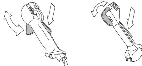
See instructions under the heading Start. Start the machine and apply full throttle. Release the throttle and check that the cutting attachment stops and remains at a standstill. If the cutting attachment rotates with the throttle in the idle position then the carburettor idle setting must be checked. See instructions under the heading Maintenance.
