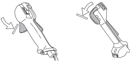
Press the throttle lockout and make sure it returns to its original position when you release it.
