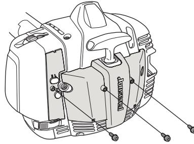
Remove the air filter and air filter cover from the machine. Fit the air filter and air filter cover supplied with the winter kit.
