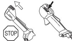
Start the engine and make sure the engine stops when you move the stop switch to the stop setting.
