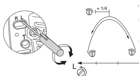
**CAUTION!** If the cutting attachment rotates when the engine is idling the idle adjustment screw T should be turned anti-clockwise until the cutting attachment stops.
