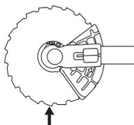
When loosening and tightening the saw blade nut, there is a risk of injury from the teeth of the saw blade. You should therefore always ensure that your hand is shielded by the blade guard when doing this. Always use a socket spanner with a shaft that is long enough to allow this. The arrow in the diagram shows the area where you should operate the socket spanner when loosening or tightening the nut.
