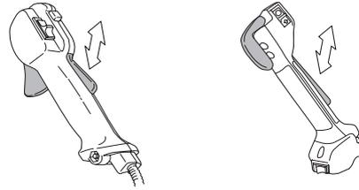
Check that the throttle control and throttle lockout move freely and that the return springs work properly.
