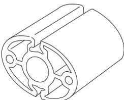
Regularly check the vibration damping units for cracks or deformation. Check that the vibration damping element is undamaged and securely attached.
