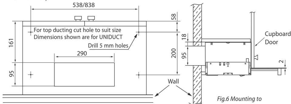
Fig.6 Mounting to underside of cabinetry
