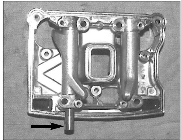
**Figure 11 - Rocker Arm Shaft Bolt Notches**
